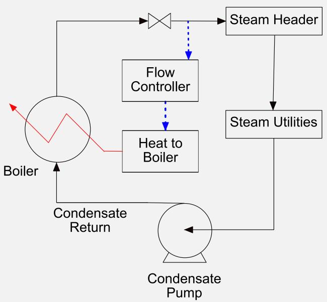
Steam is raised in a boiler and accumulates in its steam chest, before flowing through a valve into a steam utilities header. From there it is used in some sort of utilities, resulting in condensate, that is pumped back up to the boiler pressure and arbitrarily assumed to be 80 C. The condensate flow is assumed to be proportional to the holdup in the condensate tank, while a proportional integral controller regulates the heat
