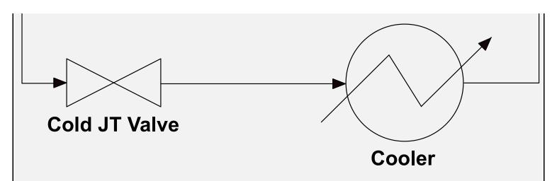
Essentially the chiller for the hot loop is the condenser for the cold loop.
