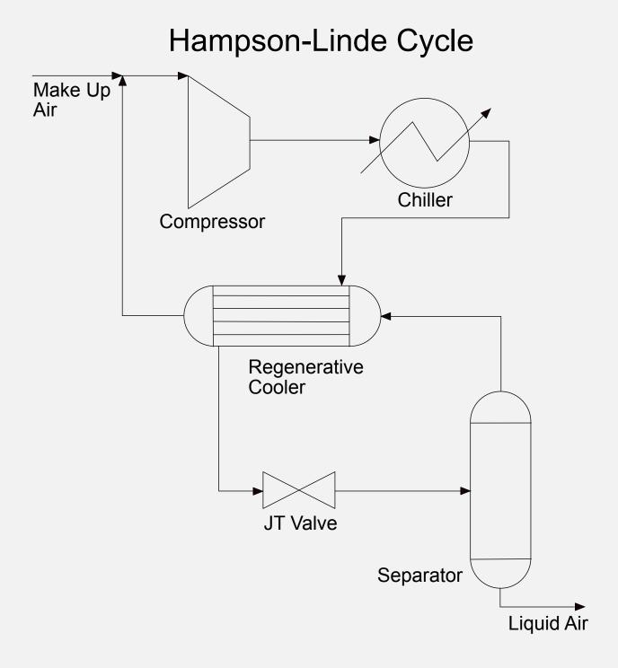
It is a pretty simple system, with air compressed to a high pressure, chilled by some external cooling, then further chilled in the regenerative cooler before being expanded to a low pressure through a valve. The Joule Thompson cooling through the valve results in partial liquification, which is the product stream. The cold vapour is passed through the other side of the renerative cooler to provide the cooling and then mixed with **MakeUpAir** before going back to the compressor.
